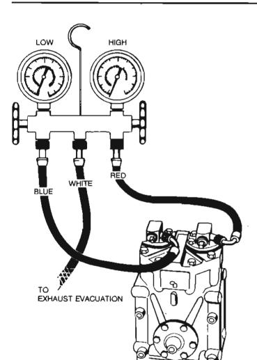
Start the vacuum pump. Open both gauge valves slowly and simultaneously.
