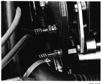
Check that gauges and hoses are correctly connected and all valves closed.
