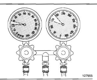
Readings at ambient temperature 20°C=68°F
