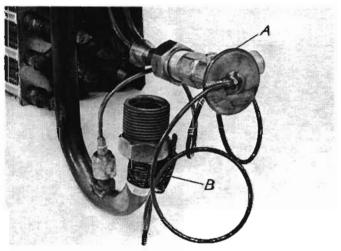
Replacing expansion valve Replace the valve (A). Attach the capillary tube (B) to the pipe.
