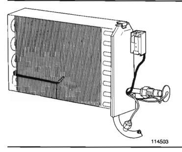
Replacing evaporator thermostat Pull the sensor out of the evaporator. Replace the thermostat. Position the sensor as shown.
