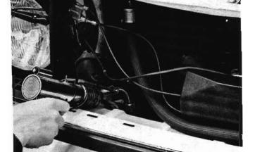
Use a leak detector to check all connections.
