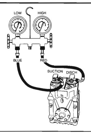
Conditions and pressures according to performance (function) test, see Specifications and Operations X1-X6.
