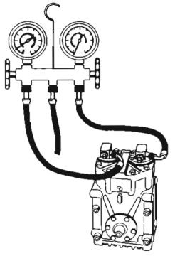
Disconnect the white hose from the vacuum pump and connect it to the refrigerant container.
