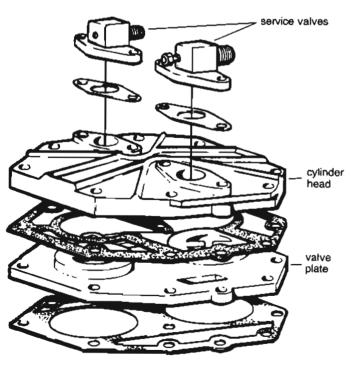
The valve plate is available as an assembly, complete with valves. It can be replaced without removing the compressor.
