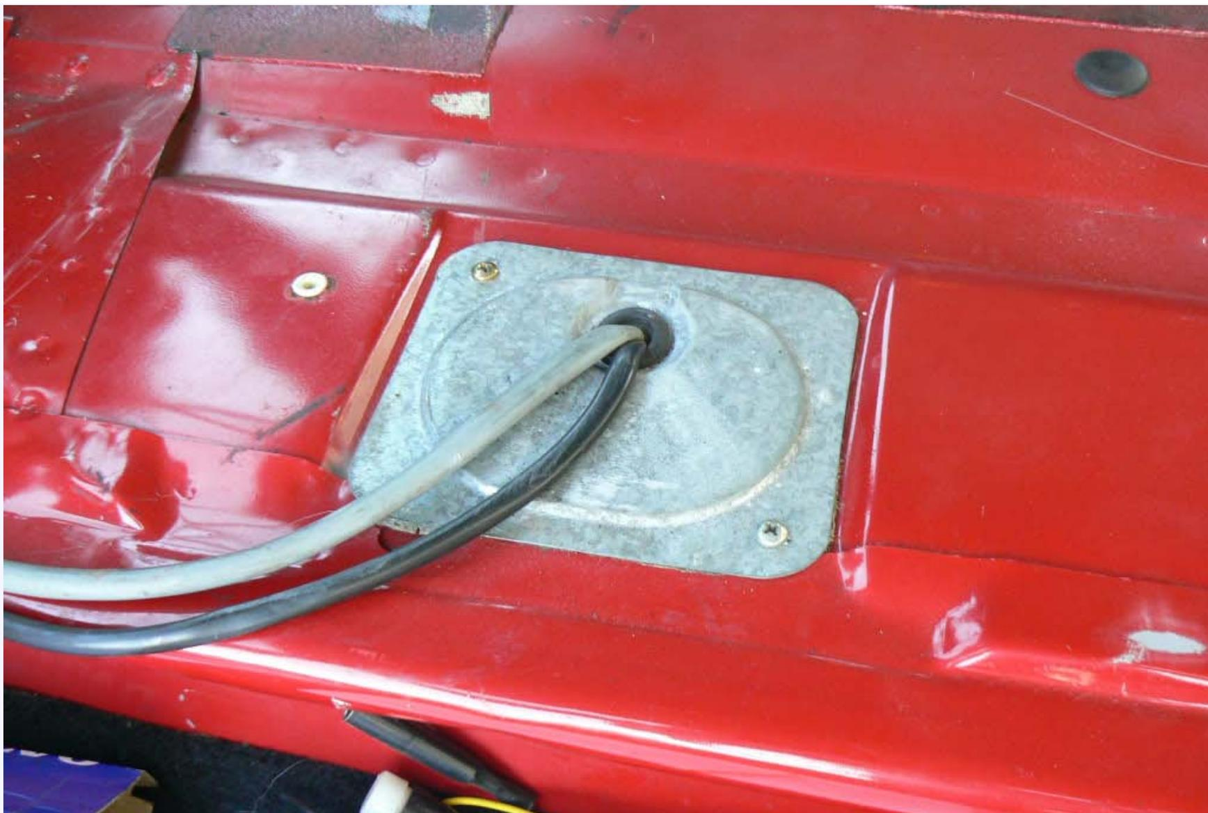
2) Unscrew the plate & slide it carefully back along the wires out of the way. Now you can see the top of the tank & the top of the sender unit with its three pipes.
