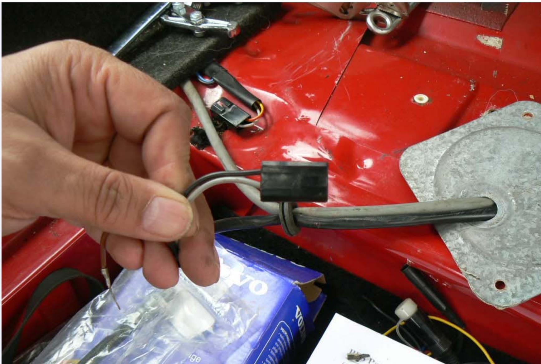
(Removing the block allows the wires to easily pass through the rubber grommit and the silver plate).
