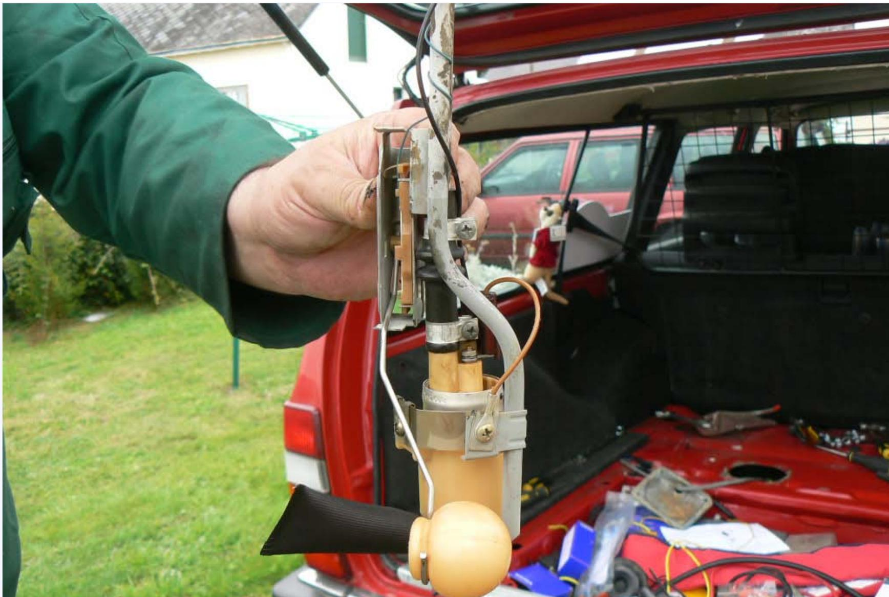
7) Now it is time to remove the dead pump from the sender unit and fit the new. This part is fairly obvious, just a case of working through it methodically. I will let the pics do the work. The sock/filter will clip off and clip back on again with a little persuasion.
