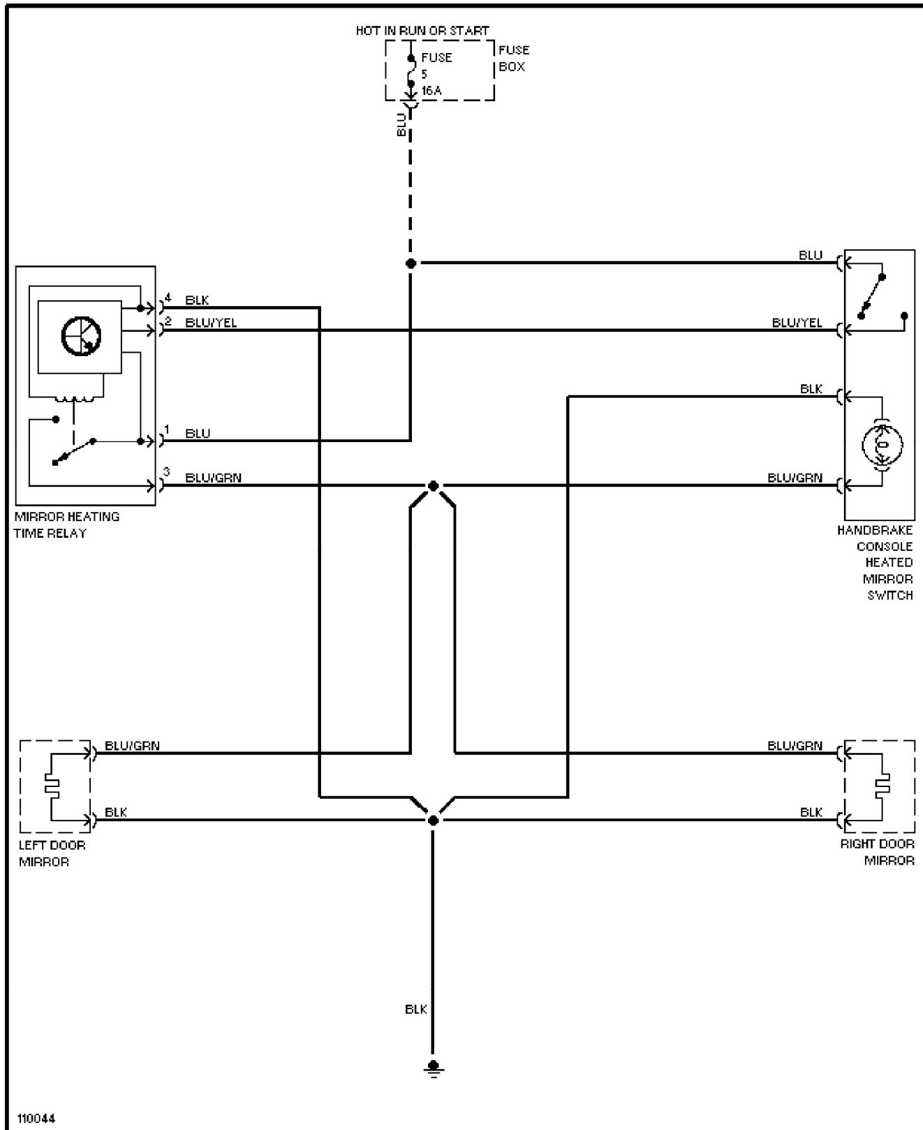
**SYSTEM WIRING DIAGRAMS**
