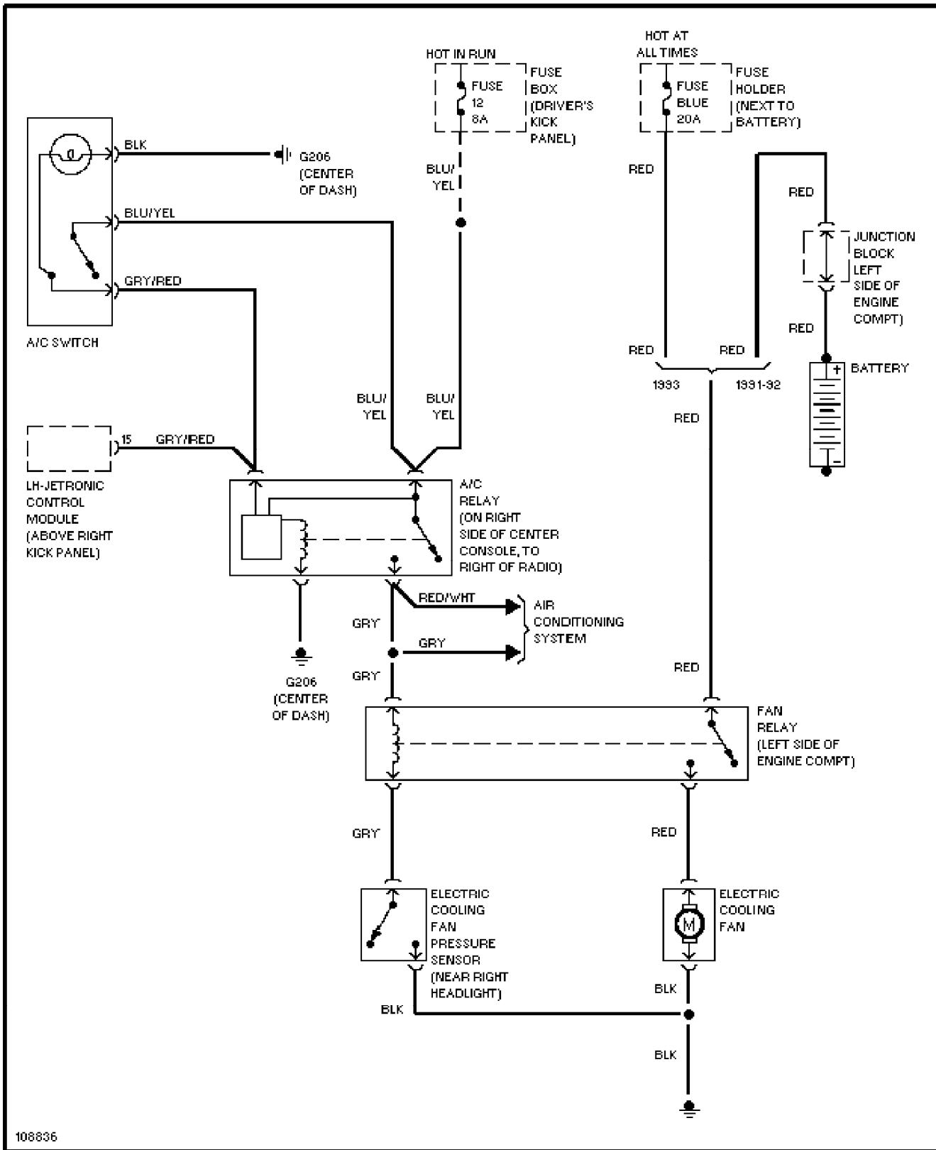
**SYSTEM WIRING DIAGRAMS**
