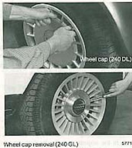
**Note:** To avoid excessive tire wear and rebalancing, mark and reinstall wheels in same location and position as before removal. To lessen the chance of imbalance, each wheel hub is equipped with a guide stud to ensure that a removed wheel can be reinstalled in its original position.
