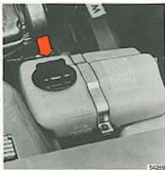
Start engine and run until hot. Check the cooling system connections for tightness. Also re-check the coolant level. Capacity: 9.9 US qts. = 9.4 liters (manual transmission models); 9.7 US qts = 9.2 liters (automatic transmission models)
