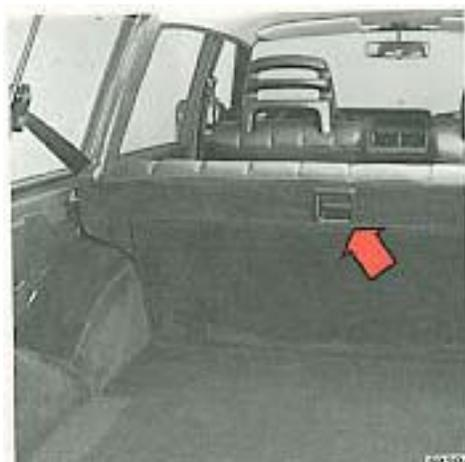
Pull the handle on the rear side of the seat back upwards, and fold the seat back forward and down so that it lies flat. The rear seat back and cushion are held automatically in their respective positions.
