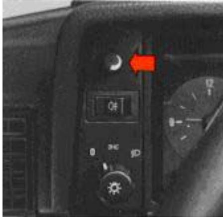
A chime will sound if the starting (ignition) key is in the switch lock when the door is open. The chime goes off when the driver's door is closed. If the headlight switch is in position
