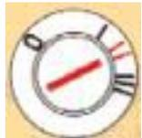
II Drive position: key position when engine is running.
