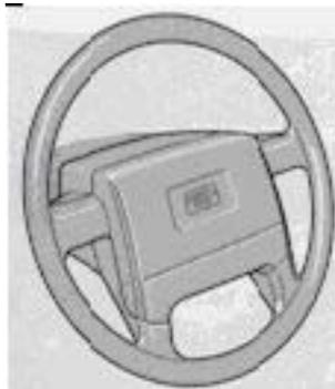
As an enhancement to the three-point seat belt system, your Volvo is equipped with a Supplemental Restraint System (SRS). The Volvo SRS consists of a drivers side air bag with a driver's side knee bolster. The system is designed to supplement the protection provided by the three-point seat belt system.
