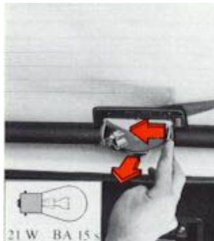
Press in reflector catch to release reflector assembly. Swing out reflector and replace bulb. Snap reflector in and check that bulb lights when brake pedal is depressed. Align the light assembly catches with the holes in the lamp housing and press it into place.
