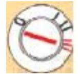
III Starting position: release the key when engine starts. The key returns automatically to drive position.
