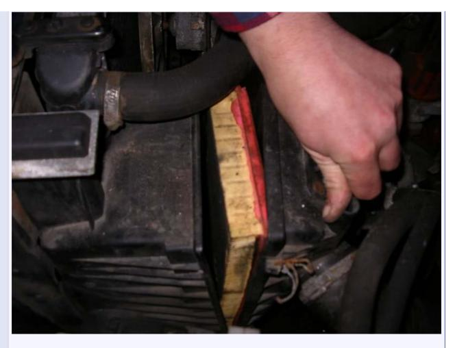
The filter can then be pulled out an d as can be seen his filter is very dirty and really overdue for change:
