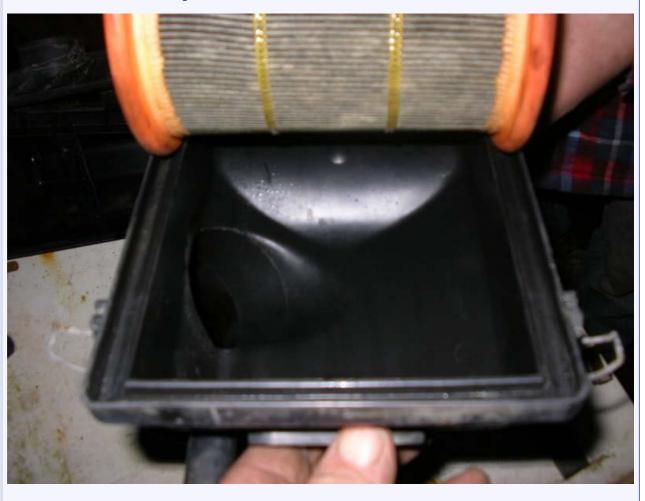
The back is slipped back at an angle into the bottom and closed up ensuring the new filter stays in position, It is then clipped into position by the two top clips:
