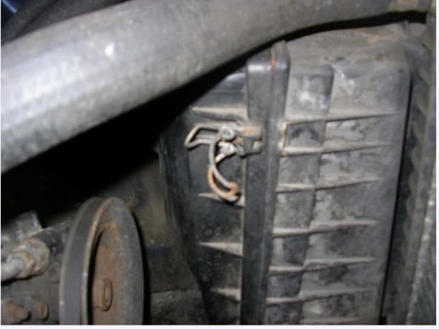
The air box will then be able to be opened by leaning the back of it towards the back of the car:  $\frac{1}{2}$
