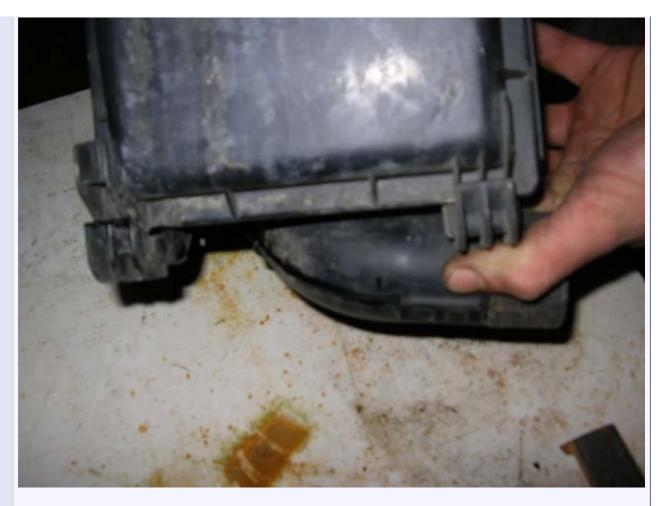
The new filter is bedded into the groove on the box itself:
