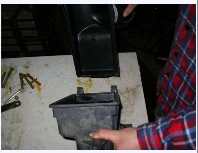
This picture shows the way the back slides down into the base to secure it:
