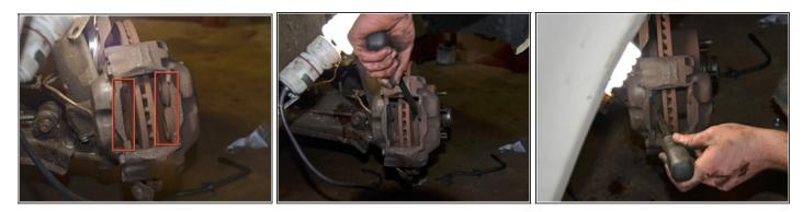
• Before installing new brake pads, you will need to compress the brake caliper pistons (shown in red) so that the pads fit inside the caliper.
