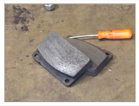
• When installing the new brake pads, make sure that they are properly seated in the caliper. If they are not, then the dowels will not go back in correctly.
