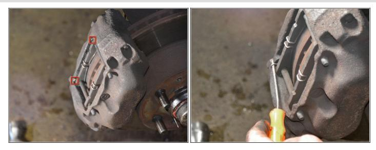
Metal clips (shown in red) hold a pair of dowels in place, which in turn hold the brake pads inside the caliper.
