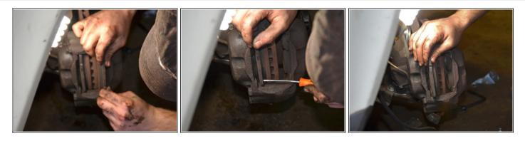
• Using your hands or a screwdriver, lift the inner and outer brake pads out of the brake caliper.
