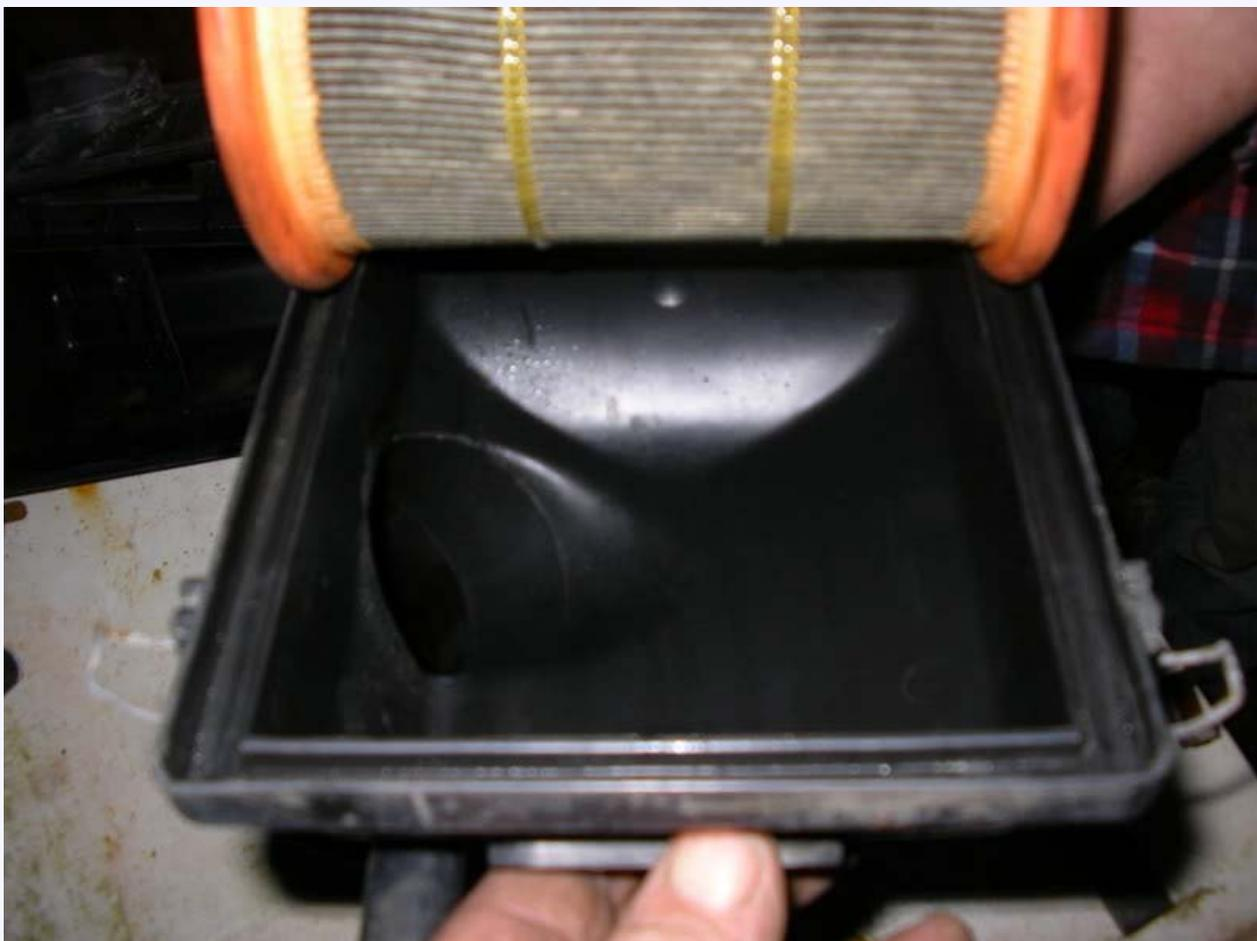
The back is slipped back at an angle into the bottom and closed up ensuring the new filter stays in position, It is then clipped into position by the two top clips:
