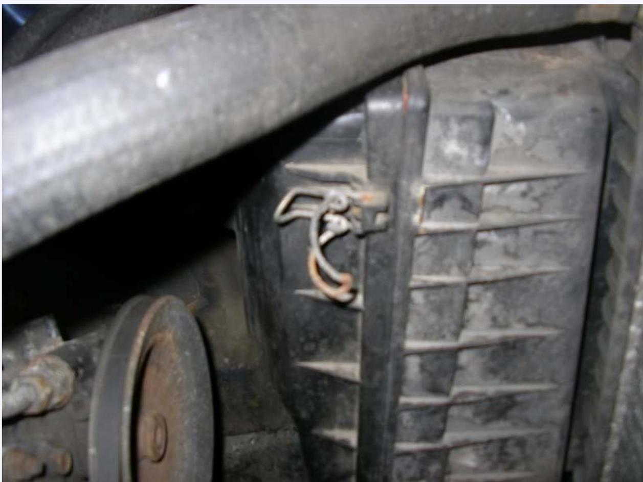
The air box will then be able to be opened by leaning the back of it towards the back of the car:
