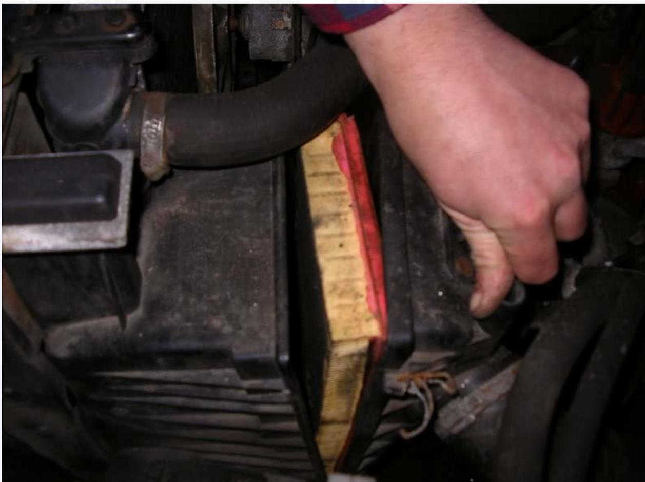
The filter can then be pulled out and as can be seen this filter is very dirty and really overdue for change:
