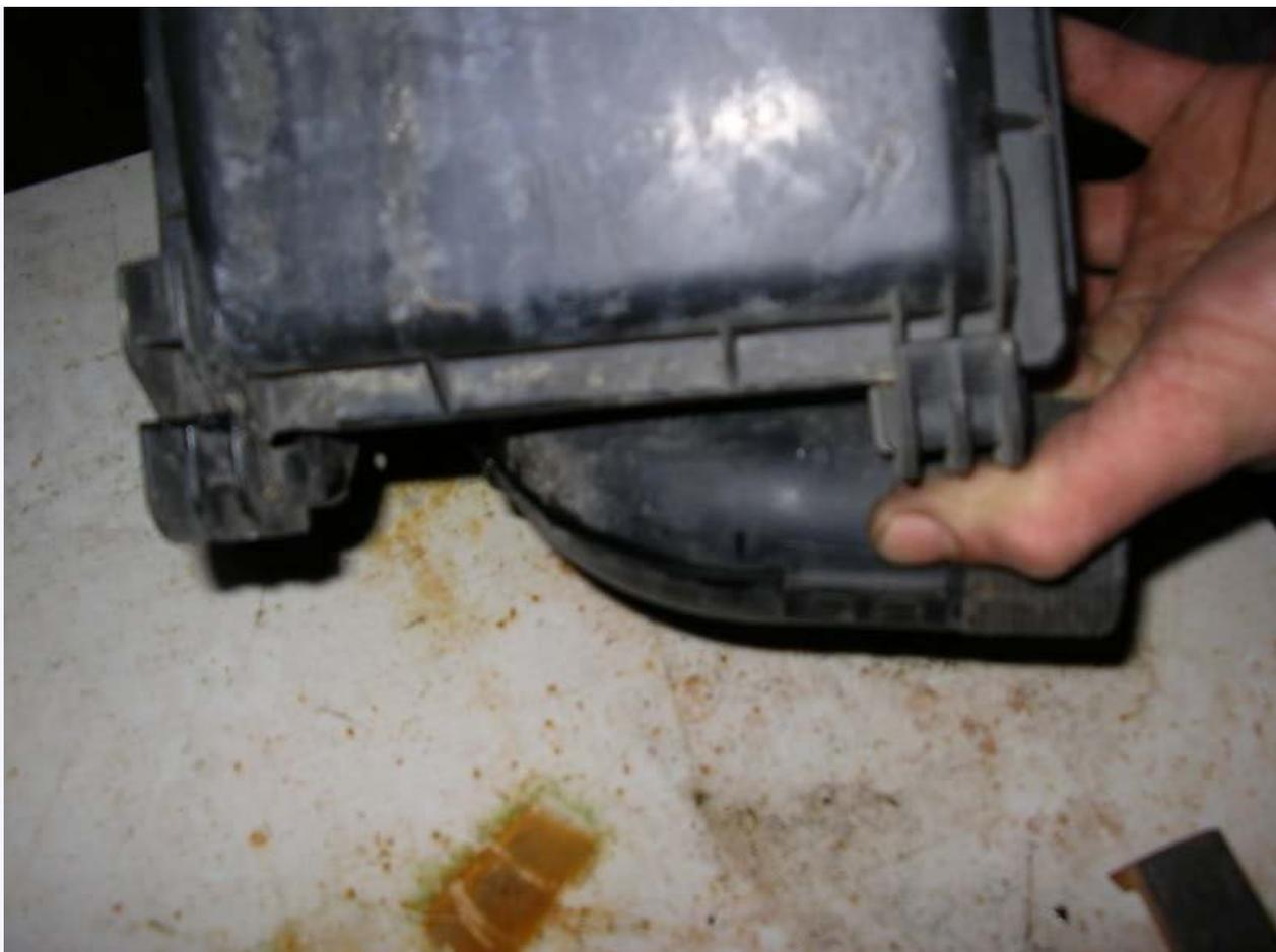
The new filter is bedded into the groove on the box itself:
