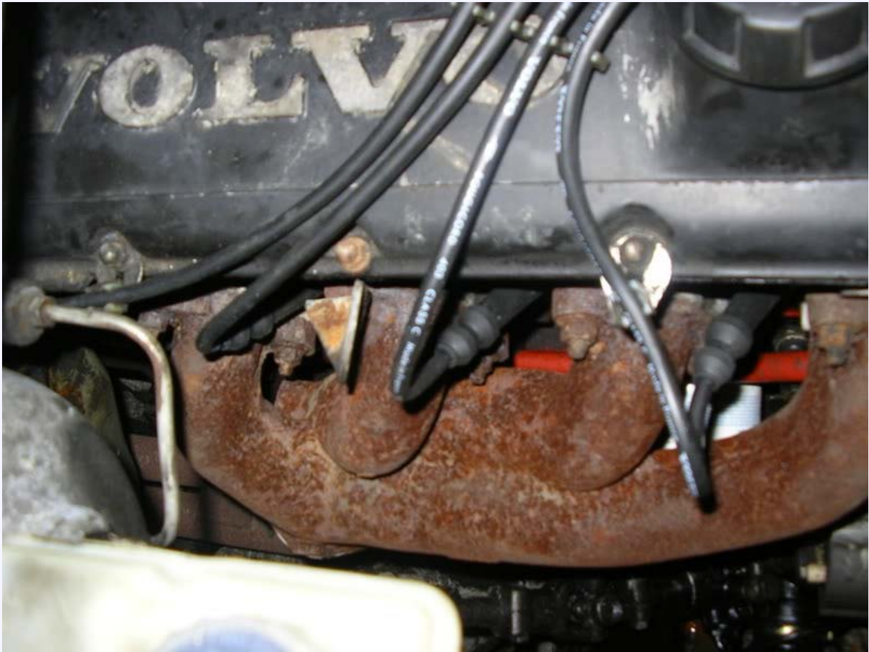
The leads should all be correctly clipped so that they cannot touch either each other or any part of the engine
