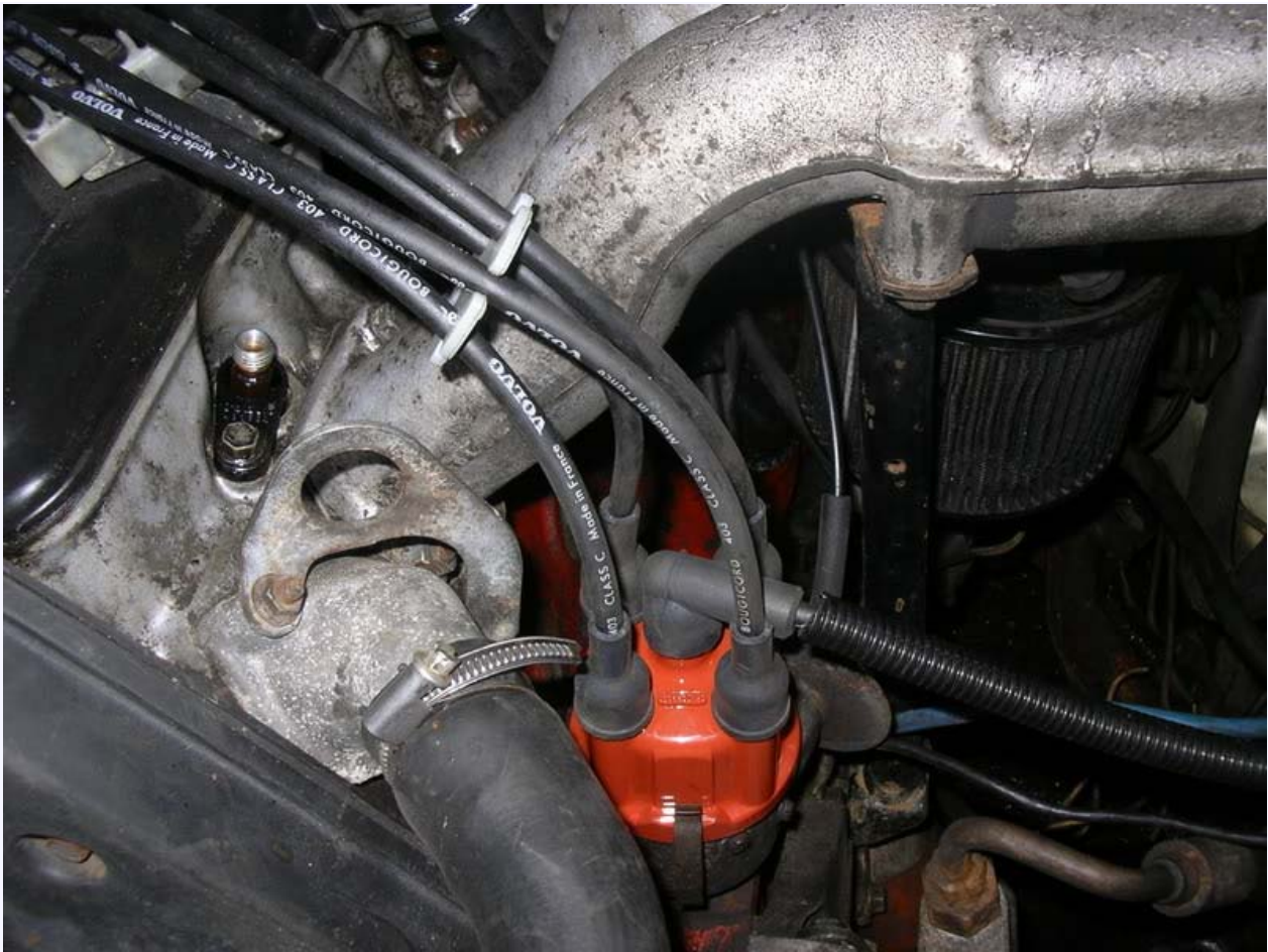
The leads should all be correctly clipped so that they cannot touch either each other or any part of the engine
