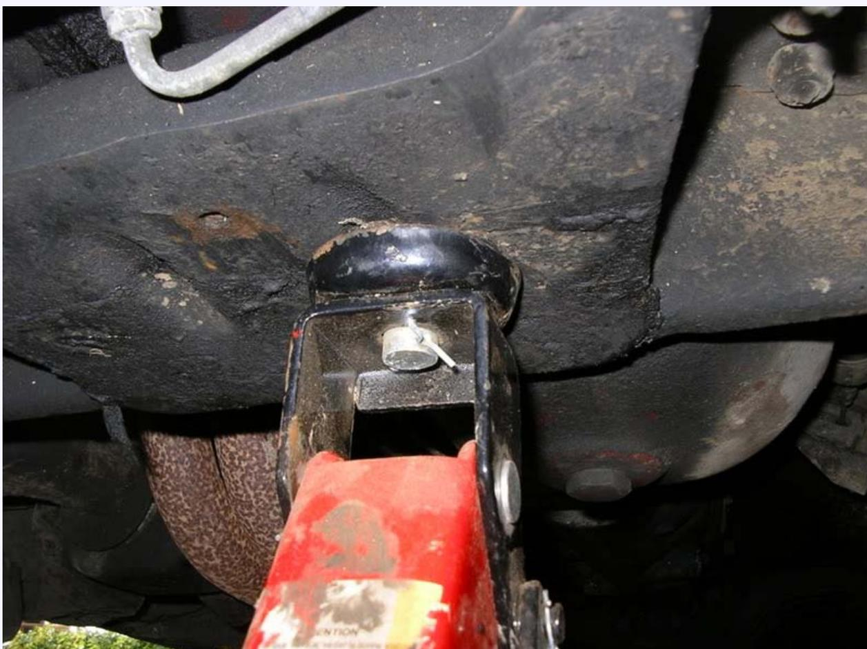
If you have a small jack the handle will be partly obstructed by the front bumper when you come to raise it meaning only short strokes can be made initially. Raise the jack up to full height. Next you will need to put the axle stand in position on the front jacking point(s) which are located behind the sill just behind the hinge of the front door. For
