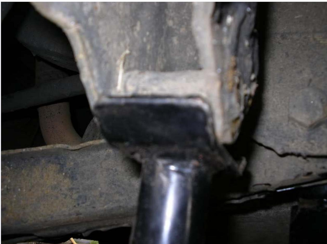
An alternative if only one side needs raising is to jack on the bracket of the trailing arm - the cup will fit on one of the brackets - use the inner one to allow room for axle stand:
