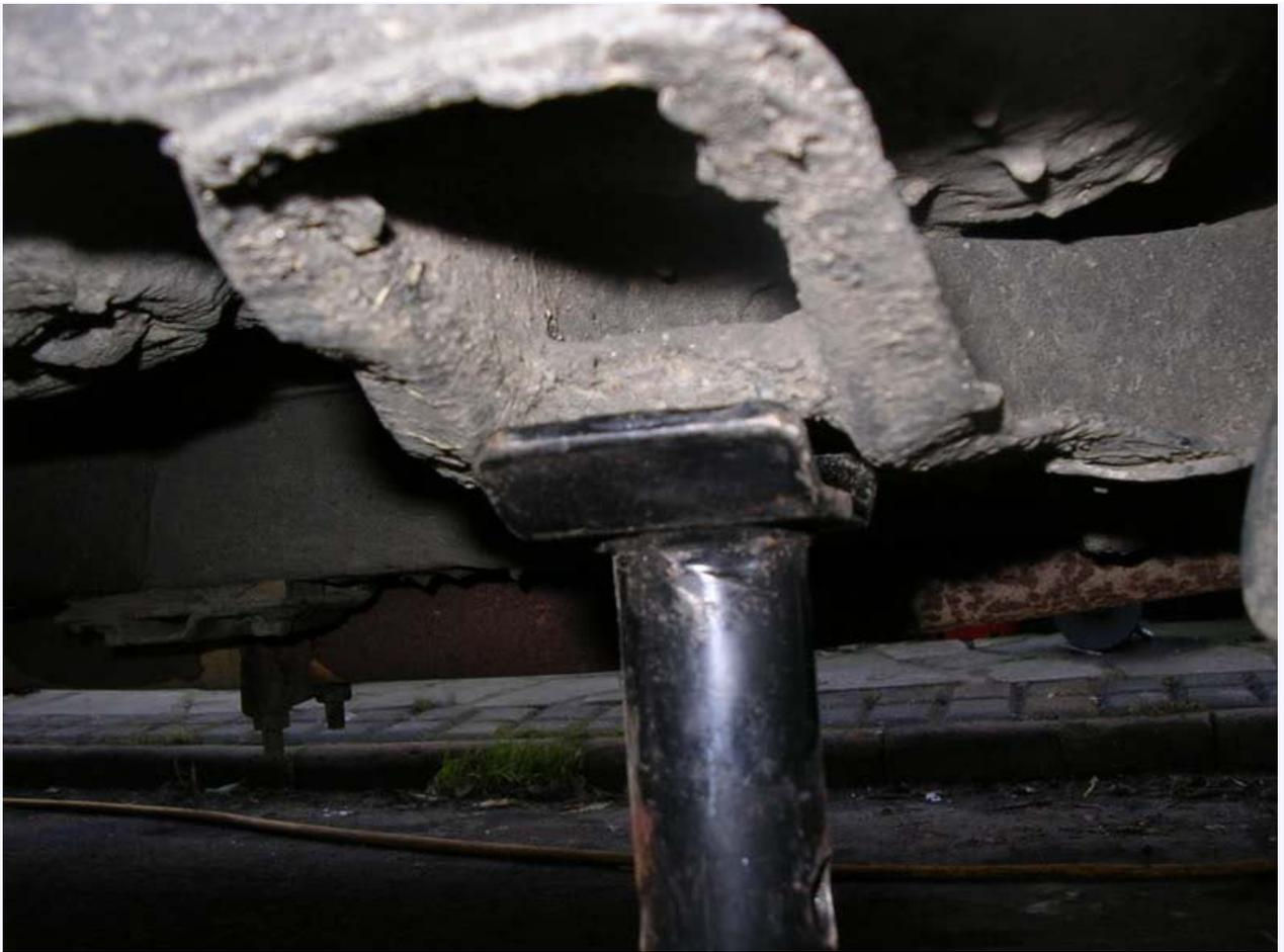
When the car is securely sat on the stands I always bring the jack back up into position (unless it will be in the way) till it again touches the crossmember so as to provide a supplementary back-up support. Never try to raise the complete car off the ground although it is ok to raise just one side. Going to the method of raising the rear - there are two possible ways. The first is similar to the front and the jack is placed under the centre of the rear axle:
