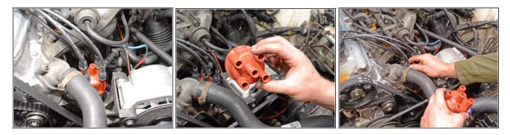
• Connect the spark plug wires to the new distributor cap one at a time. Mixing up the order will result in the engine not firing properly or at all.
