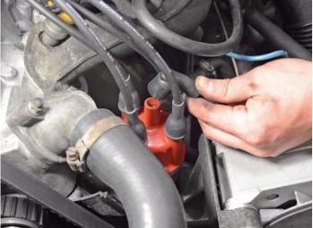
The distributor cap is located next to the engine and has all of the spark plug wires connecting to it.
