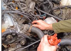
Connect the spark plug wires to the new distributor cap one at a time. Mixing up the order will result in the engine not firing properly or at all.
