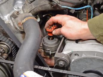
• The distributor rotor sits directly underneath the distributor cap and is not held in place by any screws or fasteners.
