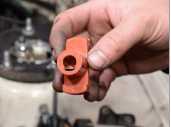
• The distributor rotor is keyed, which means that the new rotor will only go on in one orientation.
