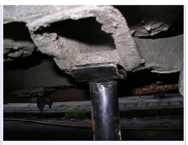
When the car is securely sat on the stands I always bring the jack back up into position (unless it will be in the way) till it again touches the crossmember so as to provide a supplementary back-up support.
