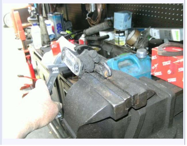
This is where we say re-assembly is the reverse order. Not quite true! Put the hinge in place and just start the two bolts into the door and then the three into the pillar. Carefully lower the door a little and tighten the bolts.
