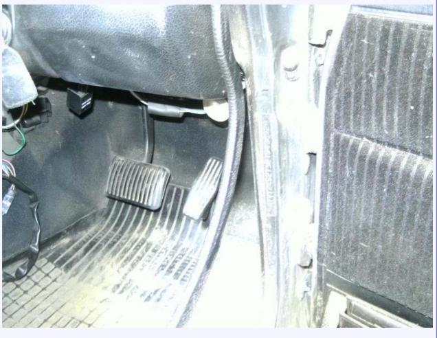
This releases the plastic cover trim. On cars with the foot vent the lever for the flap has a rubber handle with a metal pin going down through it. Push the pin out and the rubber handle will be removable. With this removed the trim can be removed.
