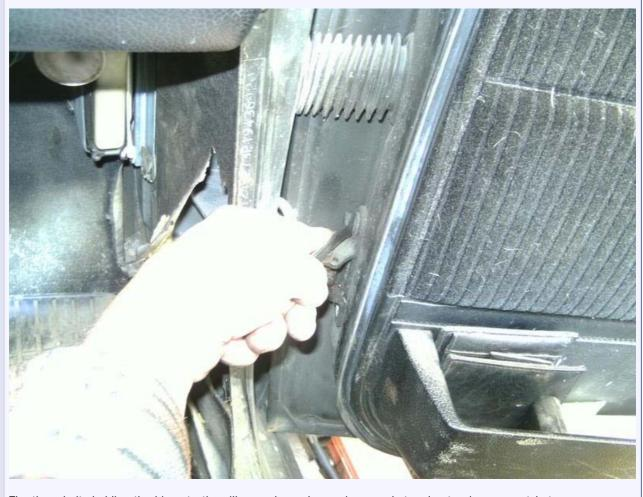
The three bolts holding the hinge to the pillar can be undone using a socket and extension on a ratchet:
