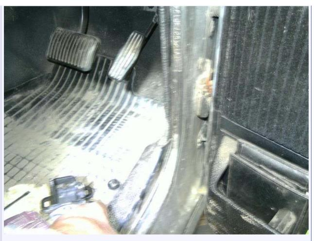
Next the trim round the frame needs removing on the hinge side - just pull away from the hinge side:
