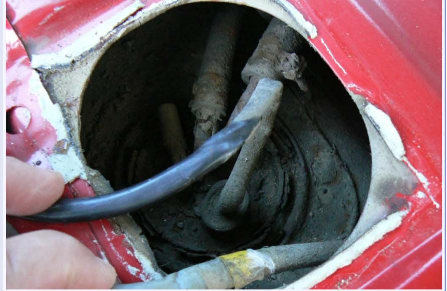
You will no doubt see lots of crud & rust flakes on top of the tank and sender unit. Get a hoover and get as much of it out as you can. You don't want it dropping into the tank later. If needs be, tape a smaller diameter tube onto the hoover pipe pipe to really get in there.
