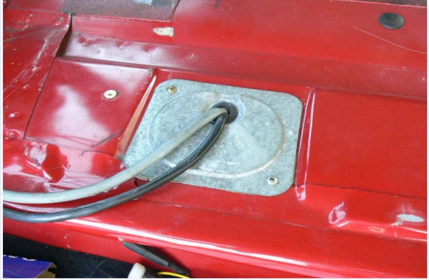
2) Unscrew the plate & slide it carefully back along the wires out of the way. Now you can see the top of the tank & the topp of the sender unit with its three pipes.
