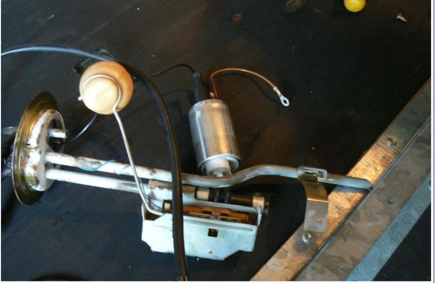
In words of the 'famous' manual, fitting the new pump is a reversal of this procedure lol.
