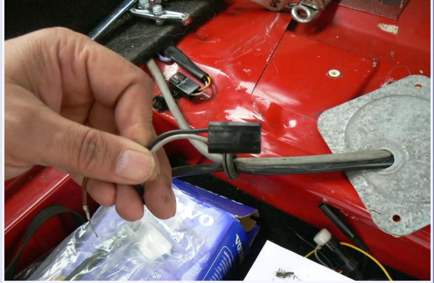
(Removing the block allows the wires to easily pass through the rubber grommit and the silver plate).
